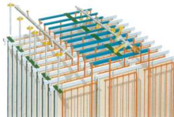
Electric corona discharge system (gas purification zones)
