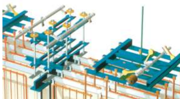
Collecting and corona discharge electrode rapping system
